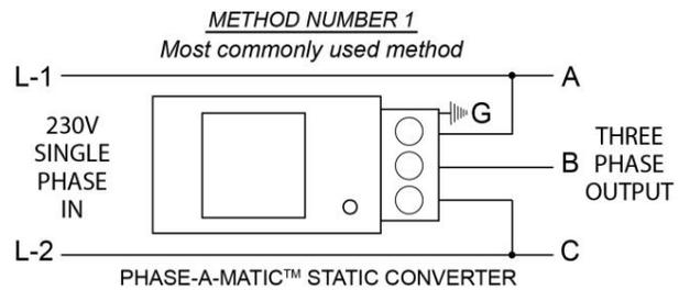
**NOTE: Mount converter upright** (vertically) with the junction box on the top. The horizontal diagram as shown here is to suit the illustration space only. It is best to mount where the red indicator light can be seen during operation of machine.
